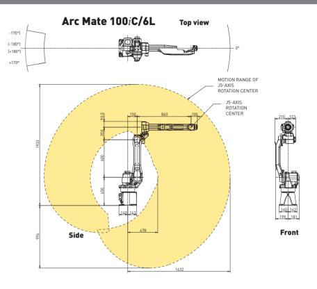
Flange Wrist Arc Mate 100iC (M-10iA Arc Mate 120iC/10L)
